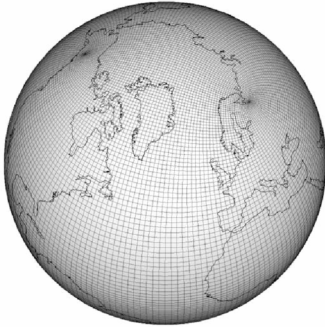
Figure 6.1. Tripolar grid. To the south of a specified latitude, the coordinate system uses latitude and longitude. To the north of that latitude, each line of constant longitude connects smoothly to a longitude line on the other side of the pair of coordinate poles. (Figure provided by Philip Jones, Los Alamos National Laboratory.)
